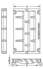
Type L vane shaped grates have the ability to remove significant amounts of sheet flow from streets, parking lots and industrial lots.
